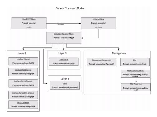
When starting a session, the initial mode is the User EXEC mode. Only a limited subset of commands are available in User EXEC Mode. This level is reserved for tasks that do not change the configuration. To enter the next level, the Privileged EXEC mode, a password is required.
